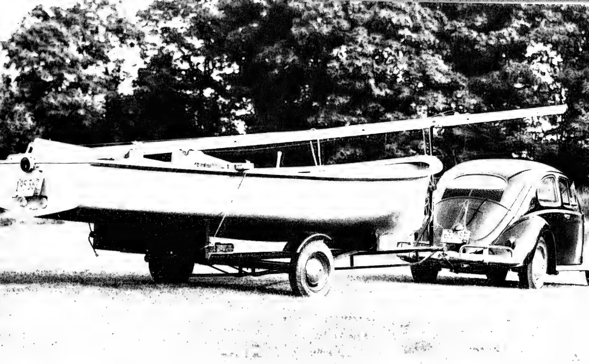
A Mobjack class centerboard boat can easily be trailed by a compact auto (top), while a special cradle is required for keel type boats such as the Amphibi-Con (bottom)
